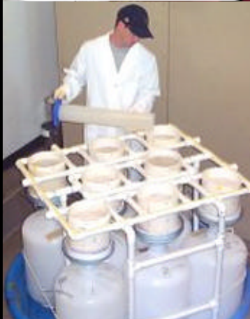
Soil column experiment for study of contaminant mobility
