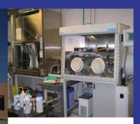
Plutonium-Glove Box in Radiochemistry Laboratory
