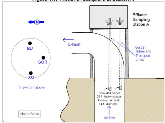
Figure 1.1: Fixed Air Samplers at Station A
