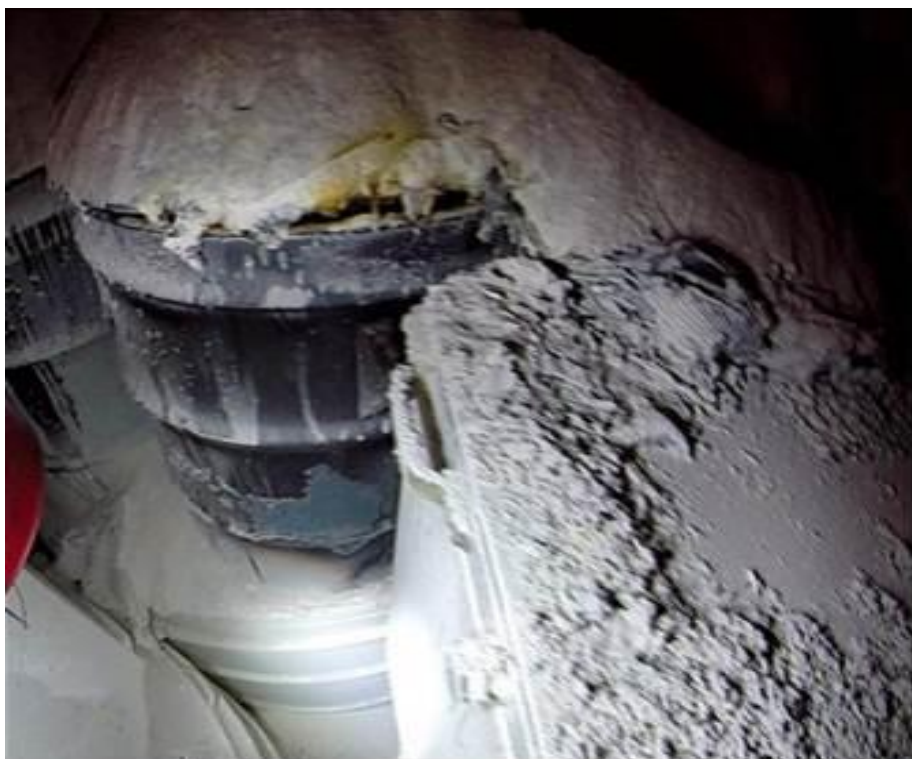
Figure 1-6: Photo of Ruptured Drum # 68660 in Room 7, Panel 7 that caused Radiation Release at WIPP
