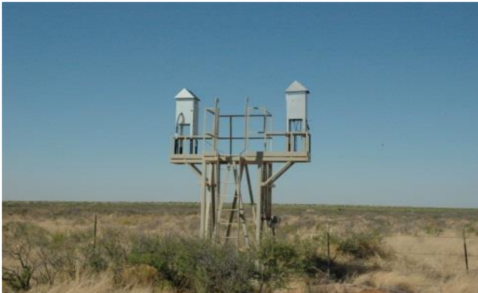
Figure 3-2: Typical WIPP Site High Volume Air Sampling Station
