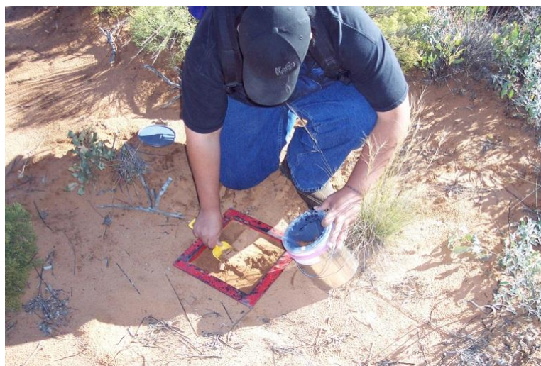
Figure 4-2: Soil Sampling in the vicinity of the WIPP site by CEMRC Personnel Sample Preparation
