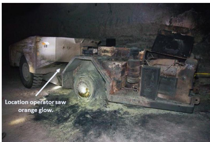
Figure 1-4: EIMCO Haul Truck 74-U-006B after Fire
