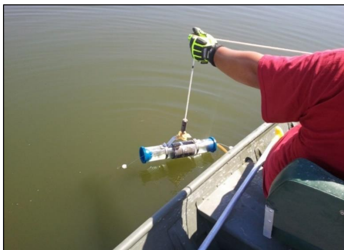
Figure 4.2. Surface water sample collection from the Brantley Lake by the CEMRC Personnel
