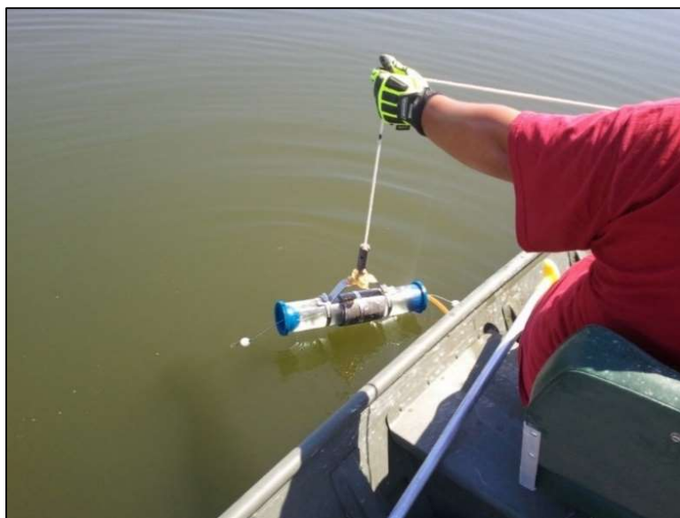
Figure 5.2. Surface Water Sample Collection from the Brantley Lake by CEMRC Personnel
