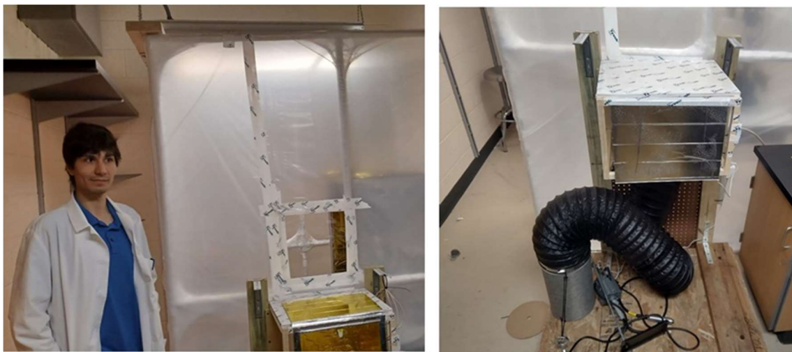
Figure 12.4. Graduate student Beowulf Owen in NMSU's new Ancient DNA laboratory, in front of the clean room constructed by him and Jeremy Winder. On the right is a close-up of the mylar-lined transfer chamber that is irradiated by UV lights and the 0.1 µm HEPA filter that interchanges the clean room every 10 minutes with HEPA-filtered air.
