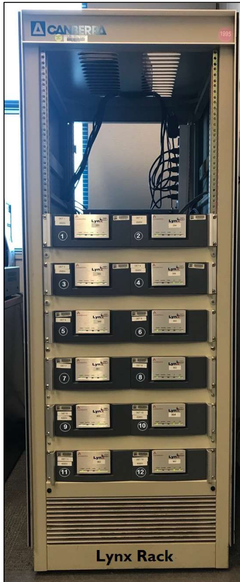
Figure 9.2. Lynx rack with twelve Lynx units mounted.
