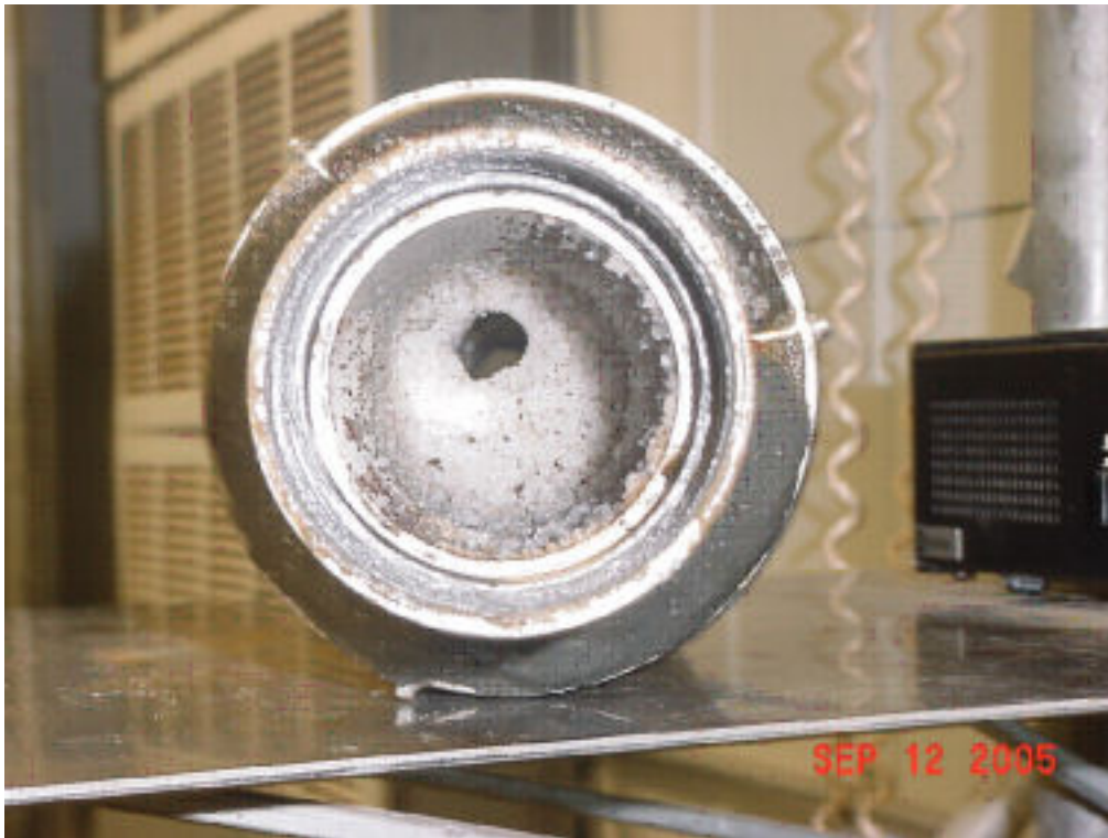
Figure 11.7: Probe Two-thirds Blocked, as Recovered (viewed from outlet side)
