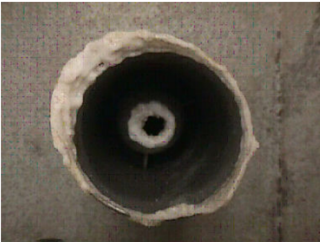
Figure 11.11: Probe Fully Occluded, as Recovered
