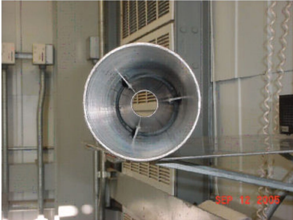
Figure 11.8: Probe Fully Occluded, Prior to Deployment
