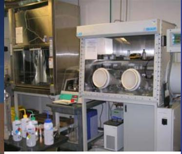
Plutonium-Glove Box in Radiochemistry Laboratory
