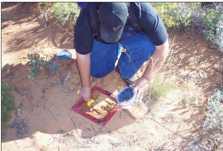
Figure 4-2: Soil Sampling in the vicinity of the WIPP site by CEMRC Personnel
