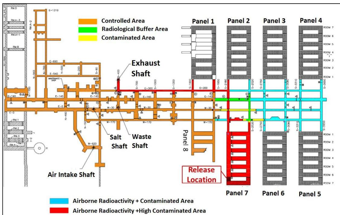
Figure 1-4: Radiological Contamination Map of WIPP Underground
