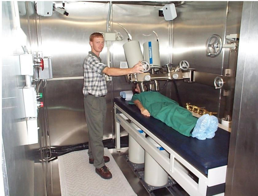
Figure 7-4: Oxygen monitor, speakers, video camera and intercom in the chamber, an operator fitting the lung detectors on a volunteer
