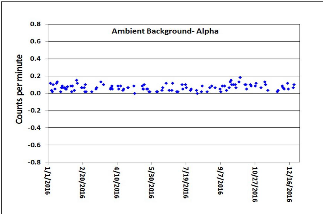
Figure 9-1: Sixty Minutes Alpha Ambient Background Count for the PIC-MPC 9604 Gross Alpha and Beta
