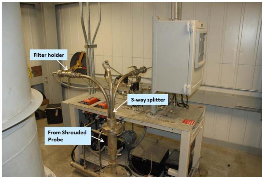
Figure 2-5: Fixed Air Samplers at Station A
