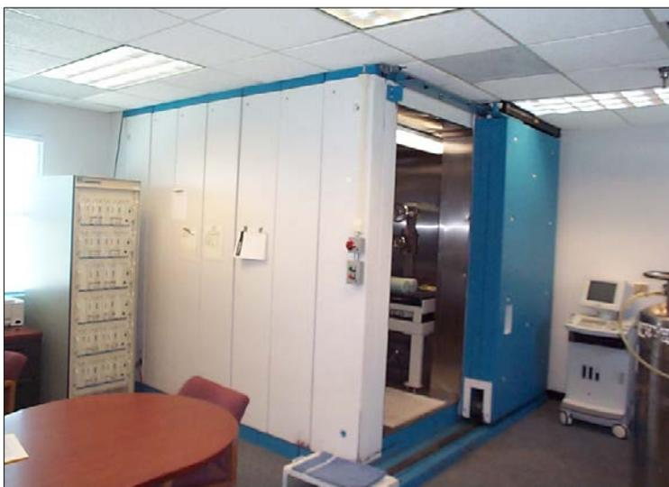
Figure 7-2: Shielded chamber for lung and whole body counting
