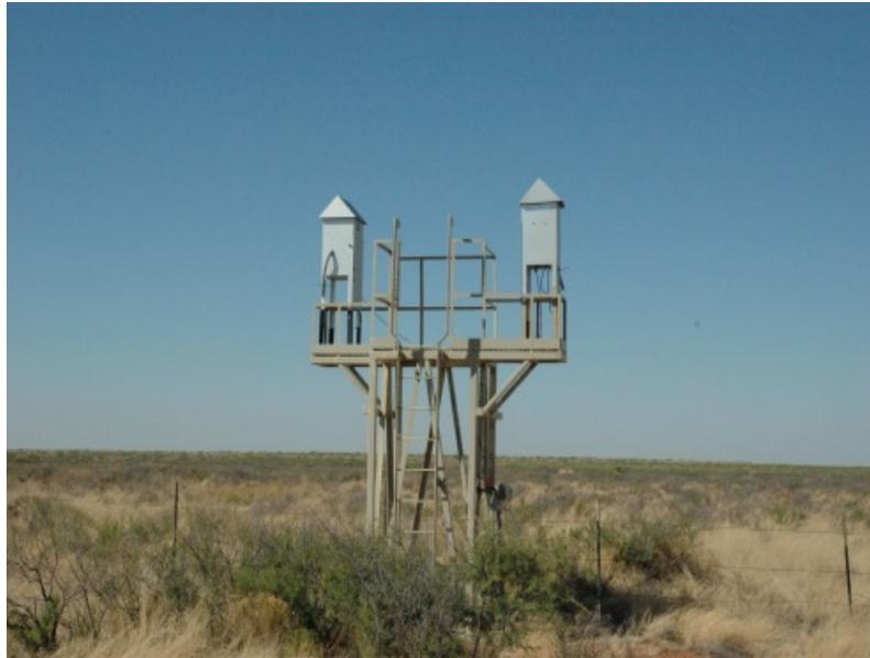
Figure 3-2: Typical WIPP Site High Volume Air Sampling Station
