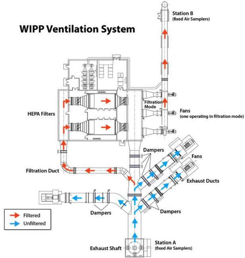
Figure 2-3: Overview of WIPP Ventilation System
