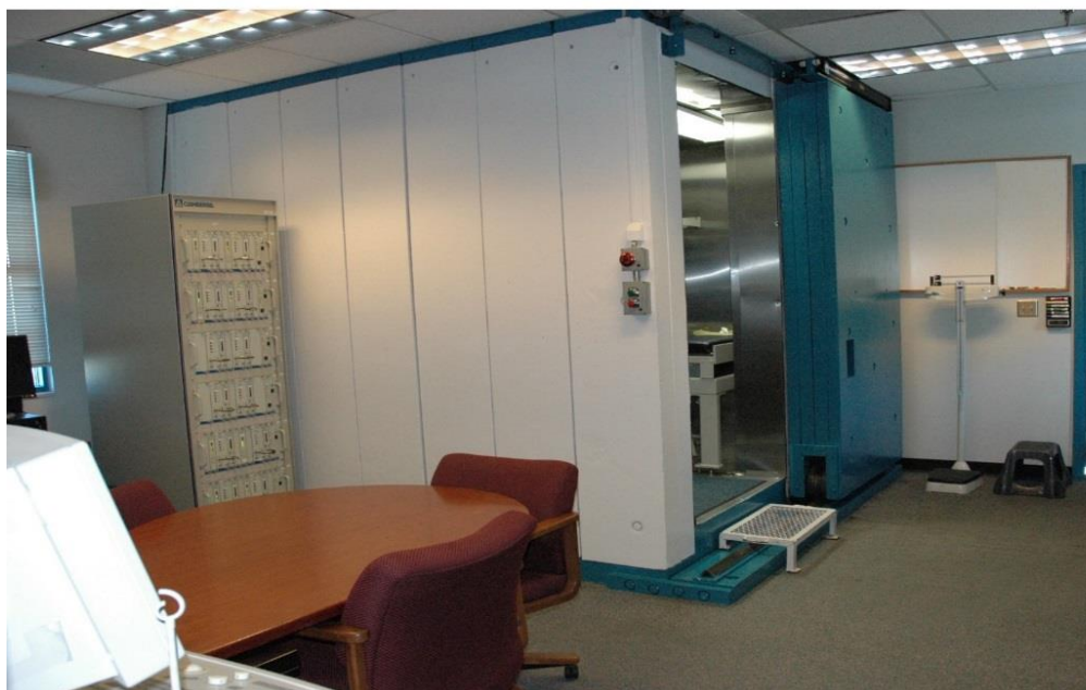
Figure 7.3. Lung and whole body counting chamber (iron wall on the side is shown in white and iron entrance door is shown in blue).
