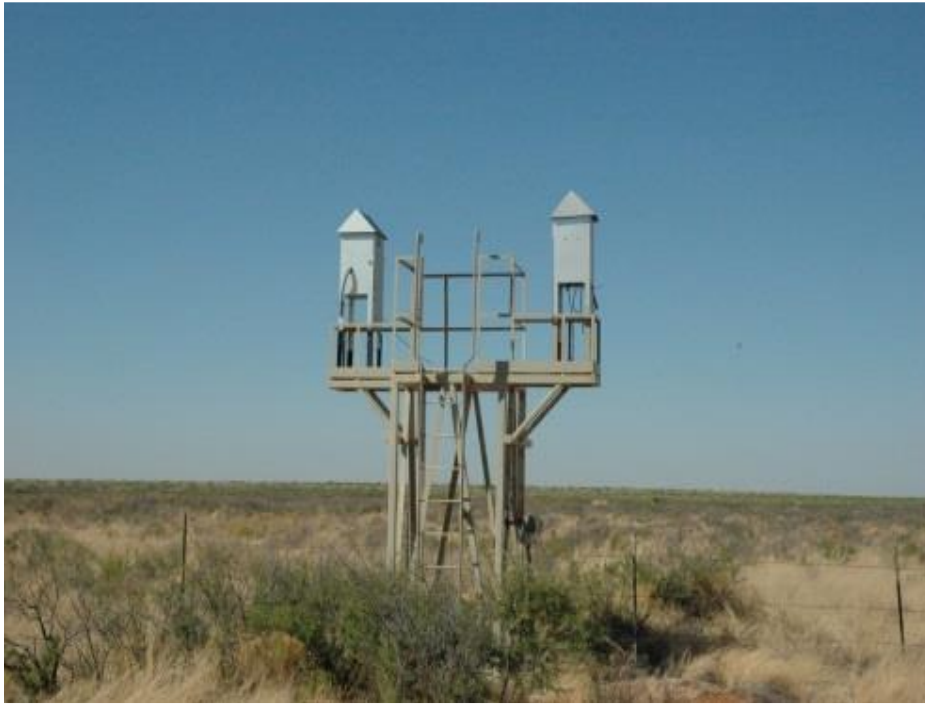
Figure 3-2: Typical WIPP Site High Volume Air Sampling Station
