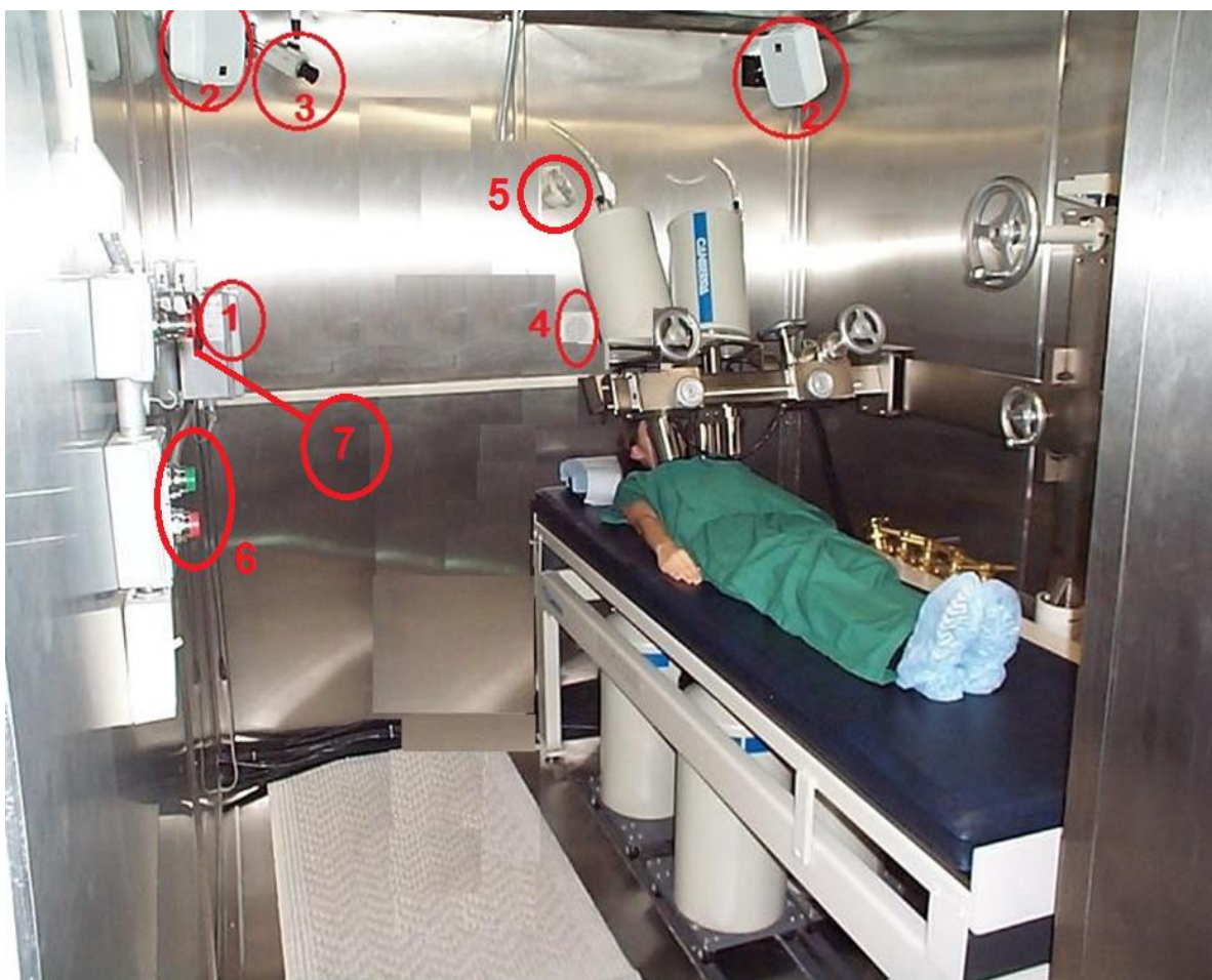
Figure 7.5. Inside the Whole Body counting chamber, (1) oxygen monitor, (2) speakers, (3) video camera, (4) intercom, (5) backup lights (6) knobs to open and close from inside, (7) emergency stop. Volunteer on the bed with lung detectors positioned on top.
