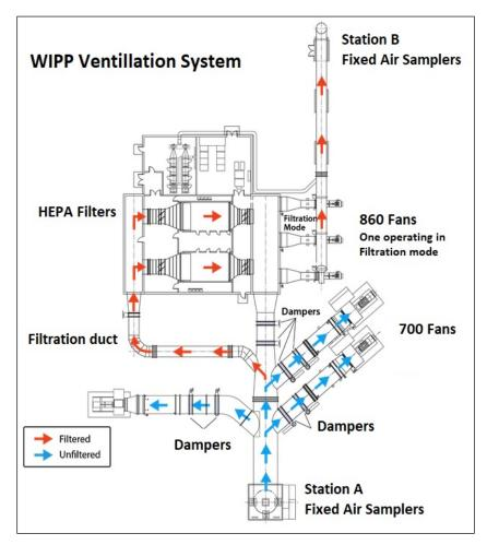
Figure 2.1. Schematic of WIPP ventilation system
