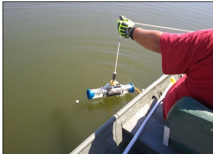
Figure 5.2. Surface Water Sample Collection from the Brantley Lake by CEMRC Personnel
